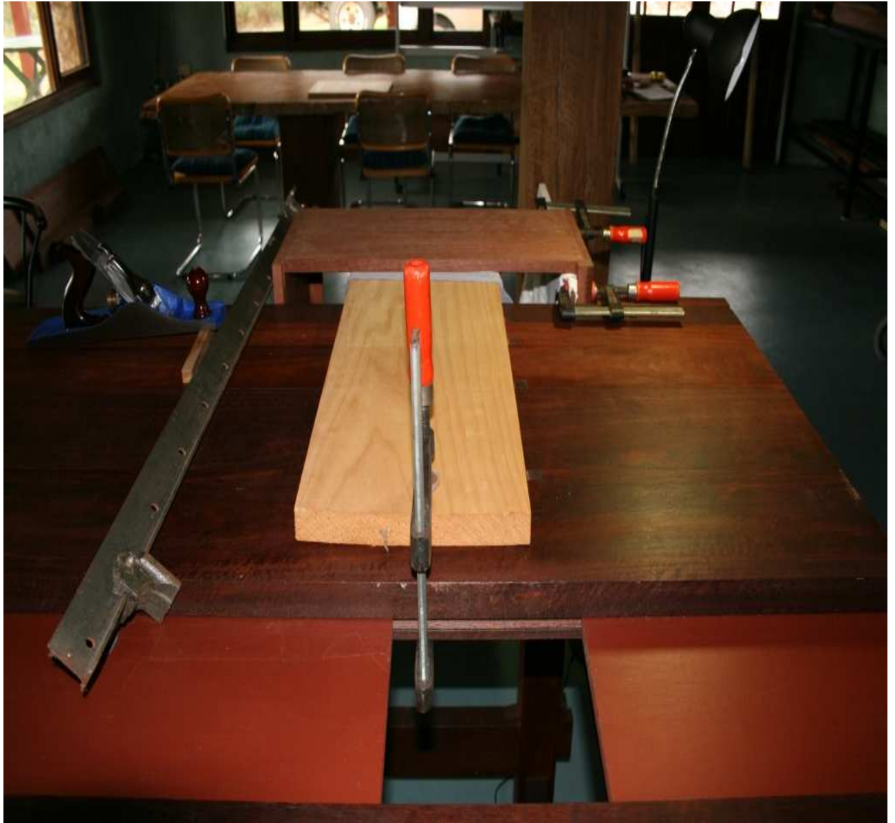
Below: The support piece to protect the end grain. A wider clamp to also clamp the middle is advisable.
