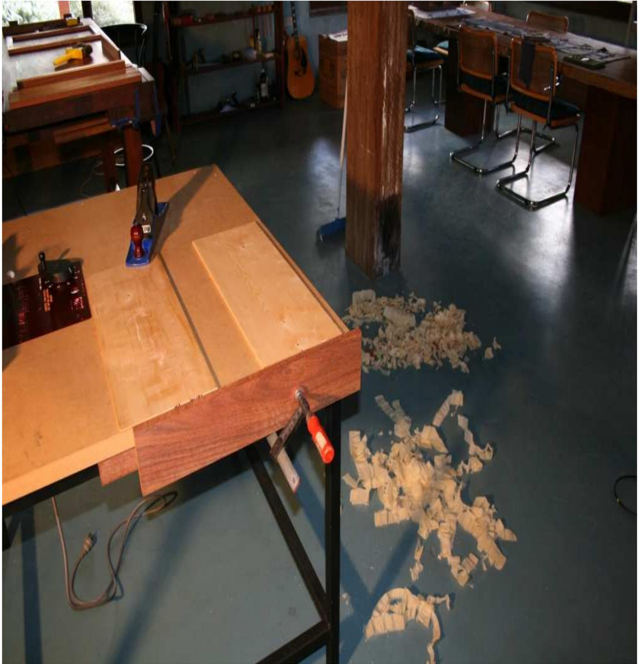
Below: Edge joining the two hand planed Huon Pine panels.
