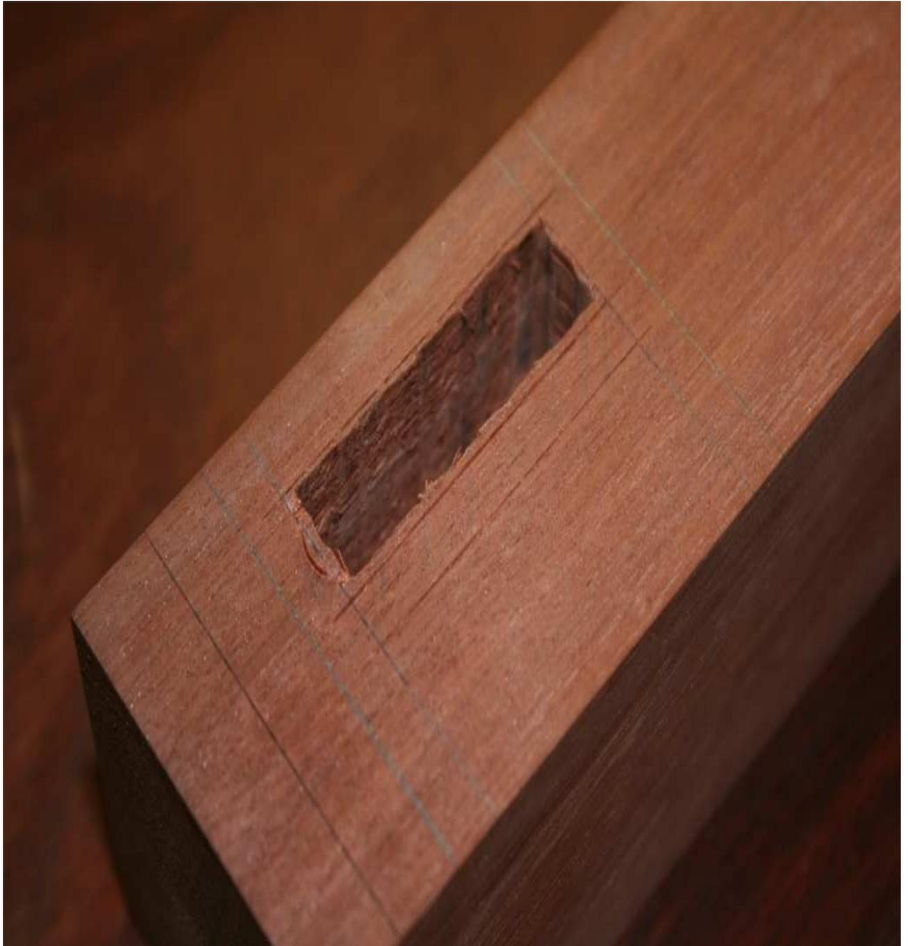
I marked the tenons out carefully using marking gauges and calipers and once again placed the rails together, clamped them, and marked out the shoulder lines so that they were consistent across all rails.
