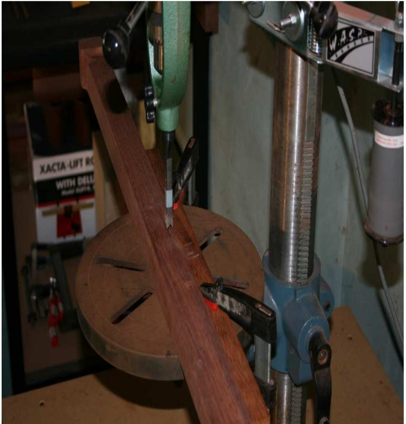
Below shows a rough cut mortise. I then chopped to the scribe line with a large and small mortising chisel and the inside faces cleaned up nicely ready for the tenon.
