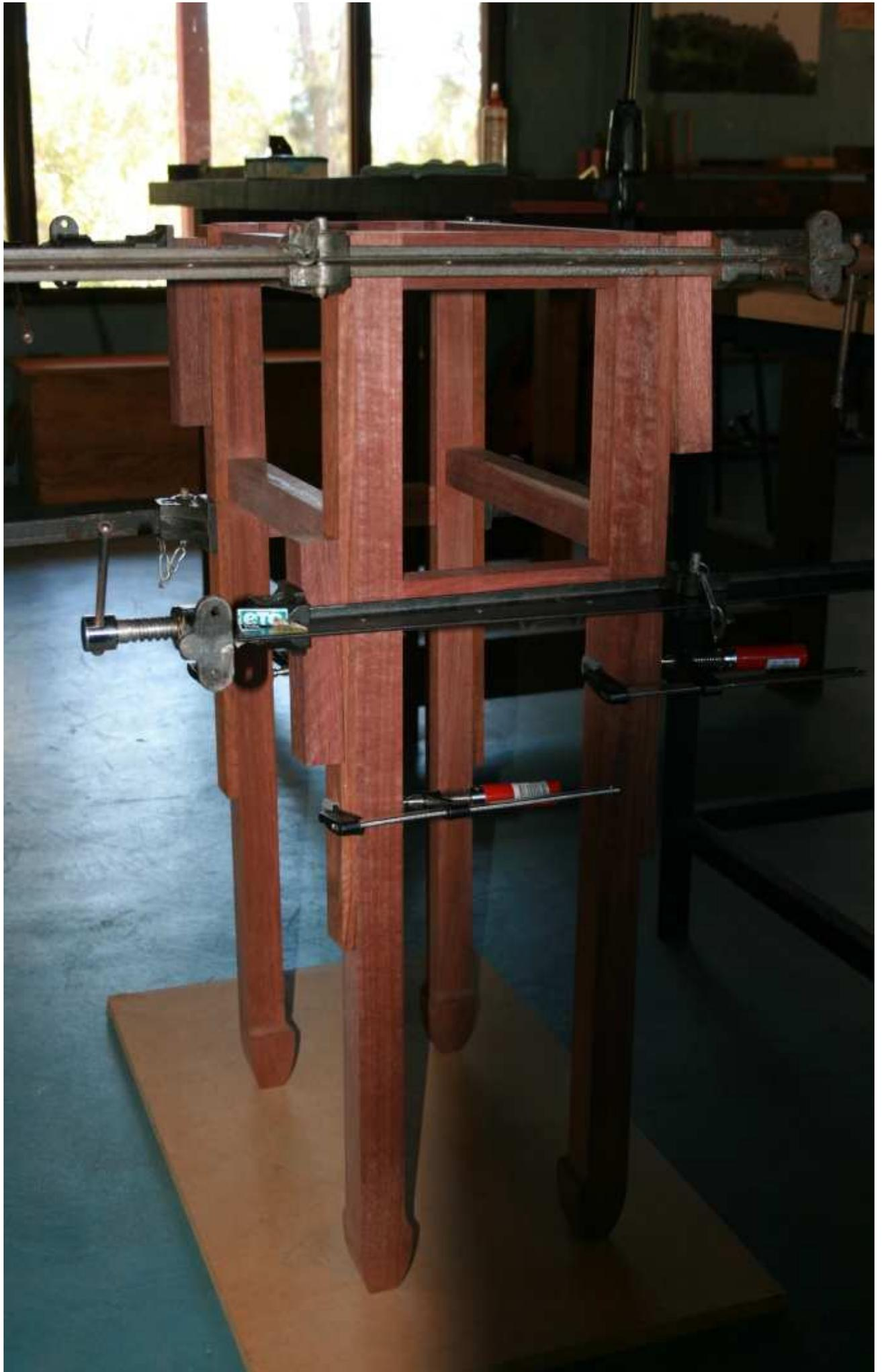
As the joinery was a firm fit I used a small paintbrush to apply a thin layer of pva glue to the walls of the mortise and the sides of the tenon. I also placed a small amount on the shoulders of the tenons. I did not want excessive squeeze out of glue and preferably would prefer none at all so that the wood surfaces around the join would remain clean cut by the handplane.
