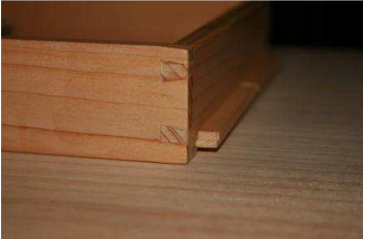
The drawer base is slid in from the back and is slot screwed into the drawer back to allow for seasonal movement. Notice how the grain runs long ways from side to side. If it ran length ways from front to back, when summer came and the wood shrank across its width, the base would pull away from the drawer sides leaving gaps along the edges where the base slots into the drawer slips.
