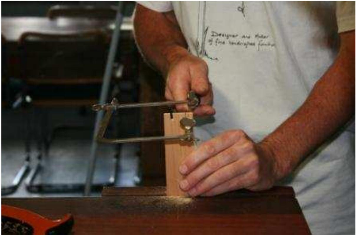
Below: A straight edged piece of wood being used as a guide to ensure accurate cutting to the gauged line.
