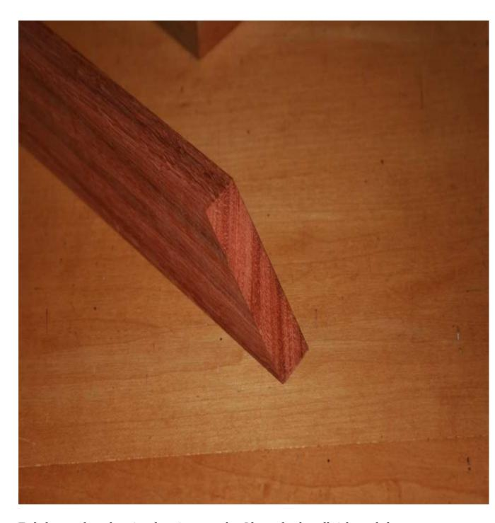
To help me when clamping the mitres together I have glued small right angled glue blocks to the long edges. These will enable me to put clamping pressure at 90 degrees to the joint and ensure a lovely, tight fit. When the frame is dry I will cut these off to within 0.5mm of the frame and then use my hand plane to remove the waste. The blocks will be gone and the frame is ready to go.
