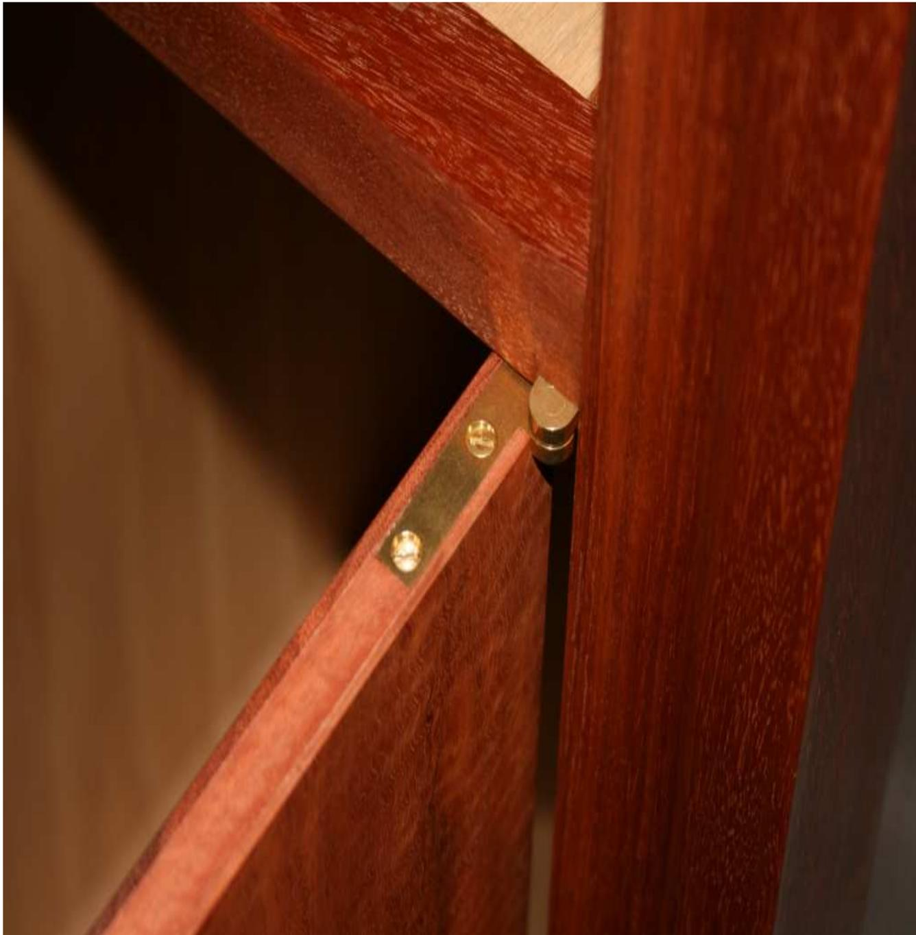
Inlaying the hinges on doors is a job for chisels. I do not take out any waste with a small hand held router as it can be difficult to balance the tool accurately. I prefer to take my time and chisel the waste out gradually until I reach the required depth. Mark out with your gauges and squares and then start to carefully remove the waste with chisels. Using sharp chisels will ensure you get crisp, accurate cuts and make the job much easier.
