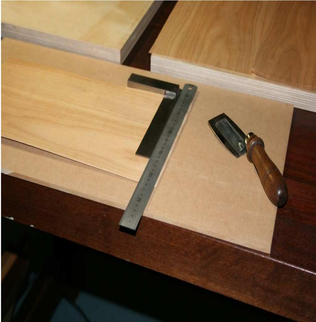
The first step in preparing the veneers is to shoot the edges where you are joining the veneers together. This was demonstrated in DVD 2. The photos below show the two veneers folded together like a book and clamped between two pieces of hardwood/(Jarrah). The edges are protruding out from the edge of the jarrah by only 2mm so that edge can be planed. If you protrude the edge too much the veneer may bend and prevent you from cutting a clean, straight edge.
