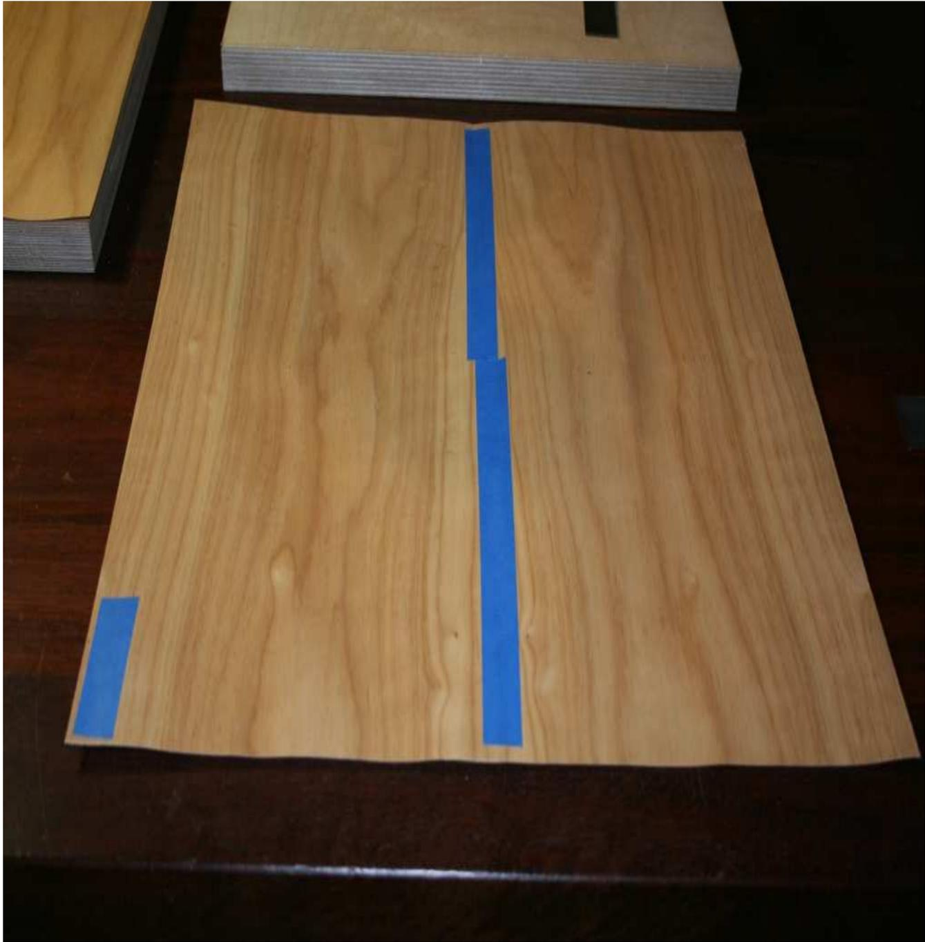
Once you have taped them together you can turn the piece over and have a look at the 'show face' and see how tightly the edge join has pulled together.
