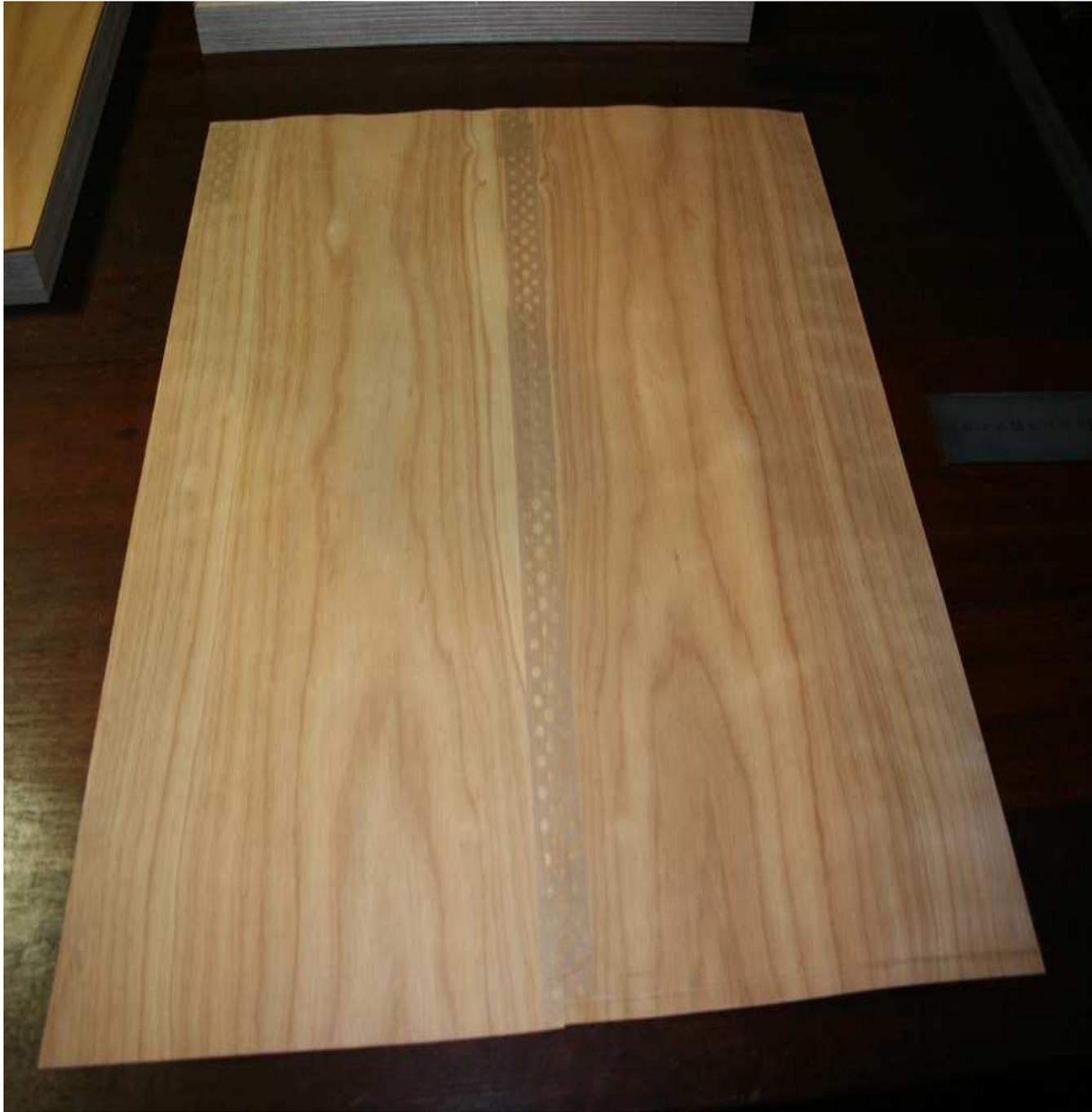
Turn the piece over and carefully remove the blue tape from the surface to be glued.
