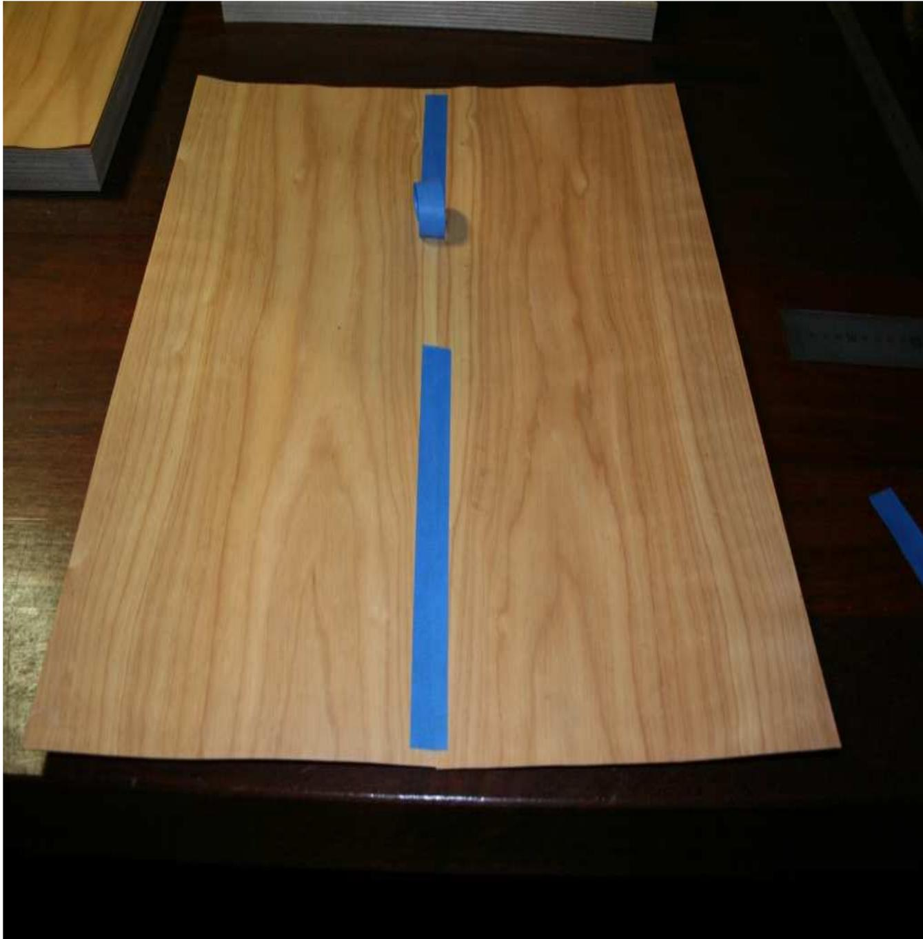
You are now ready to glue the veneer to the substrate material. The substrate material I am using in the sideboard is White Birch Multiply (WBM). I am using Better Bond Cold Press Veneer Adhesive as the glue to bond the two together. I use a roller to apply an even coat of glue to the substrate. I then place the veneer carefully onto the substrate and cover the veneer with newspaper. Then I cover the top surface with two pieces of 16mm mdf and place as many clamps as possible.
