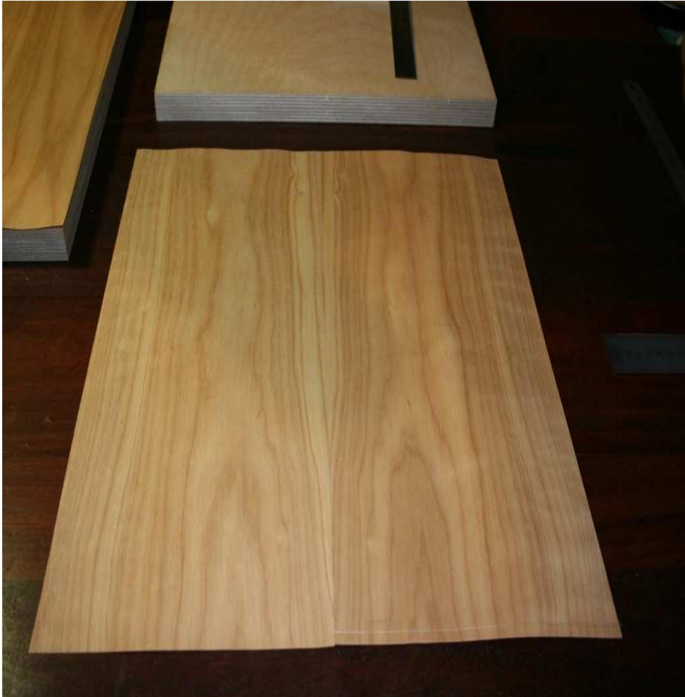
If you are happy with your join you can then tape the 'show surface' using the stronger light tan coloured veneering tape. This tape needs to be slightly wet before placing onto the veneer. Once you have taped the 'show surface' you can then safely remove the blue tape from the surface to be glued to the substrate.
