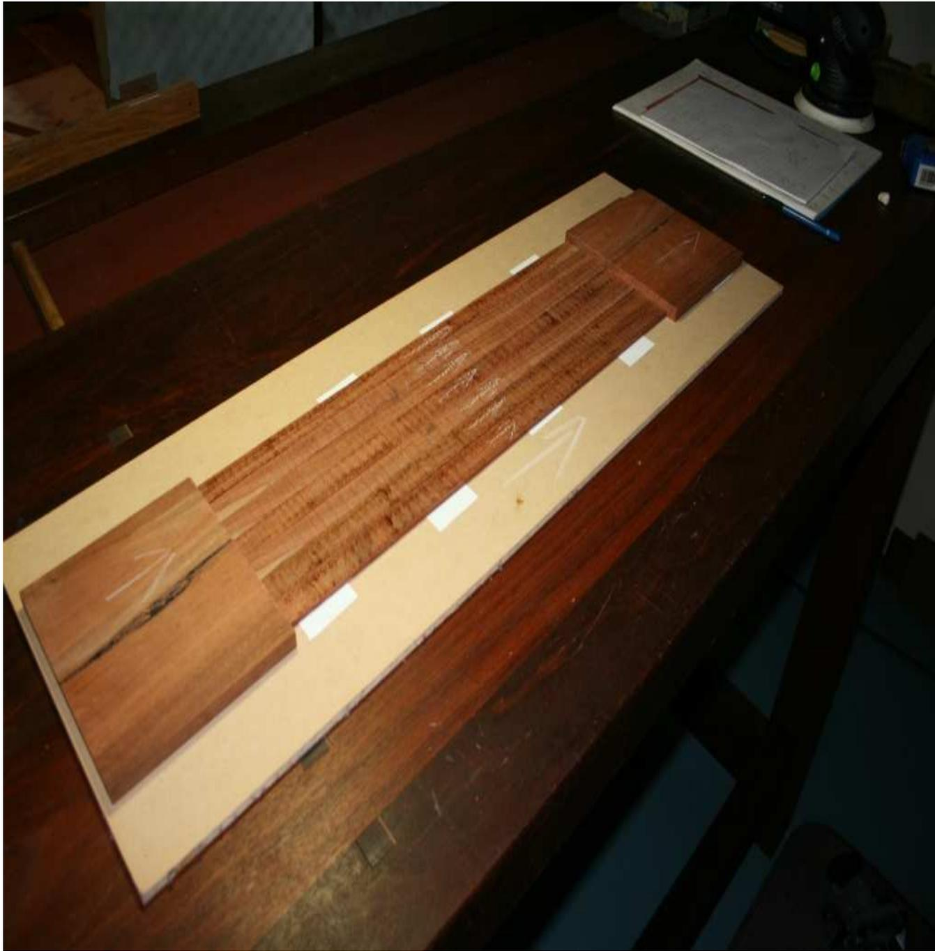
I have used double sided tape to stick all of the strips to a piece of 8mm mdf. At each end I have also stuck some thicker pieces of Jarrah. I have ensured that the grain direction on all pieces runs in the same direction. When I run this through the thicknesser the first piece of jarrah will take the initial shock of the rollers before the blades pass onto the Ironwood.
